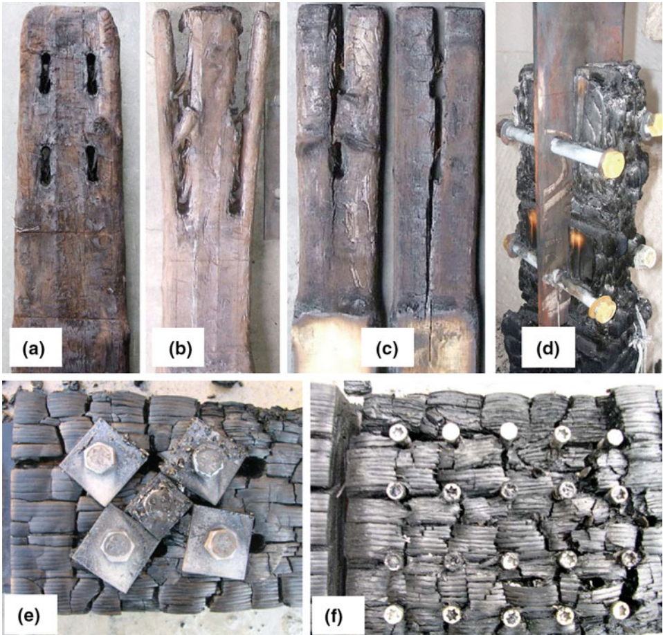
Figure 13. Failure modes of heated WSW connections tested by Peng et al. [15] (a–d) and Lau [16] (e, f). (a)–(d) Reprinted with permission of Multi-Science Publishing Co Ltd. Copyright© 2012 Journal of Structural Fire Engineering.
