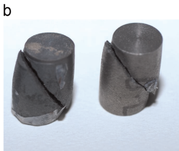
Fig. 12. (a) Ambient temperature stress-strain diagrams of cast iron (Group F and H tests) and (b) shear failure mode of Group H specimens.
