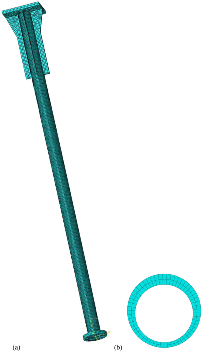
Fig. 5. (a) Finite element mesh of an unprotected cast iron column (No. 9) (34040 elements); (b) finite element mesh for the cross-section.
