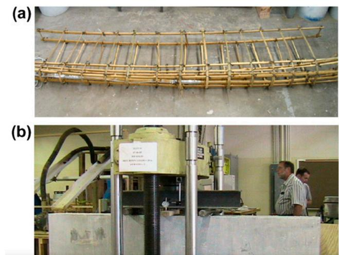
**Figure 11.** Concrete beams reinforced with bamboo rebars: (a) finished reinforcement, (b) the setup [51].
