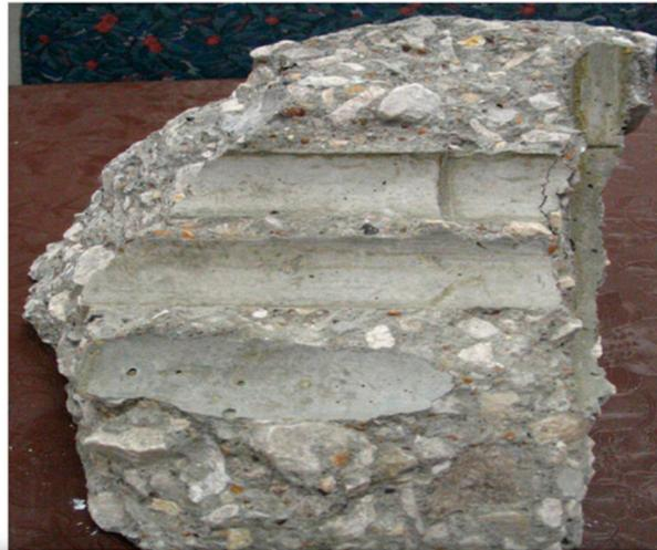
**Figure 12.** Imprint of bamboo reinforcement in cementitious material [51].
