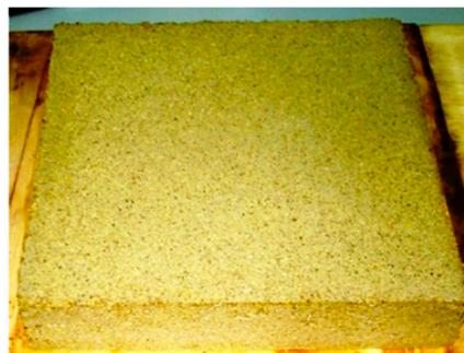
Figure 7. Lime–hemp mixture in insulation panels [42].
