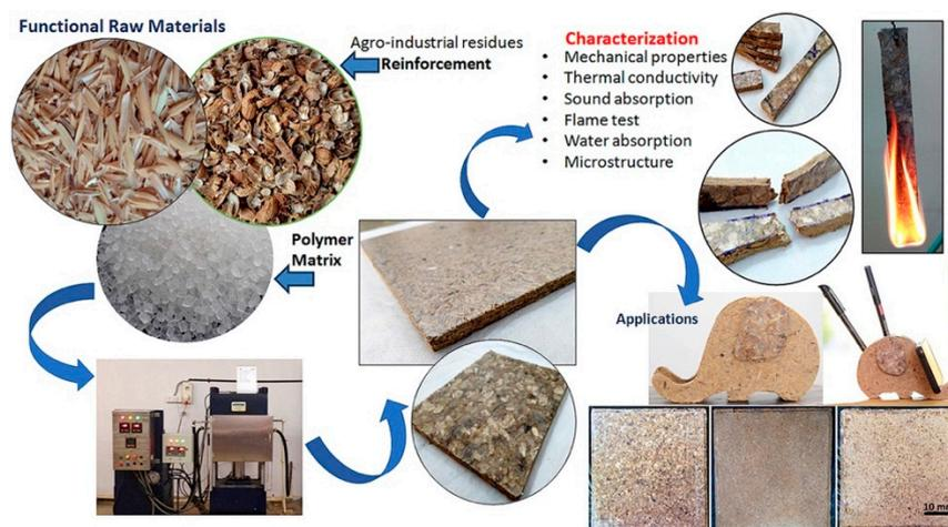
**Figure 13.** Reinforcement of hybrid polypropylene using rice husk and groundnut shells [3].
